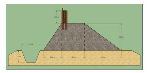
Figure 4. A view of the defence mound model with wooden structure and a water moat
